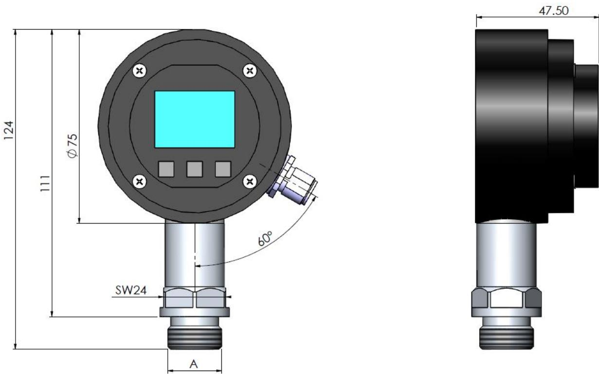
\* Dimension A is the thread dimensions on the pressure sensors.
