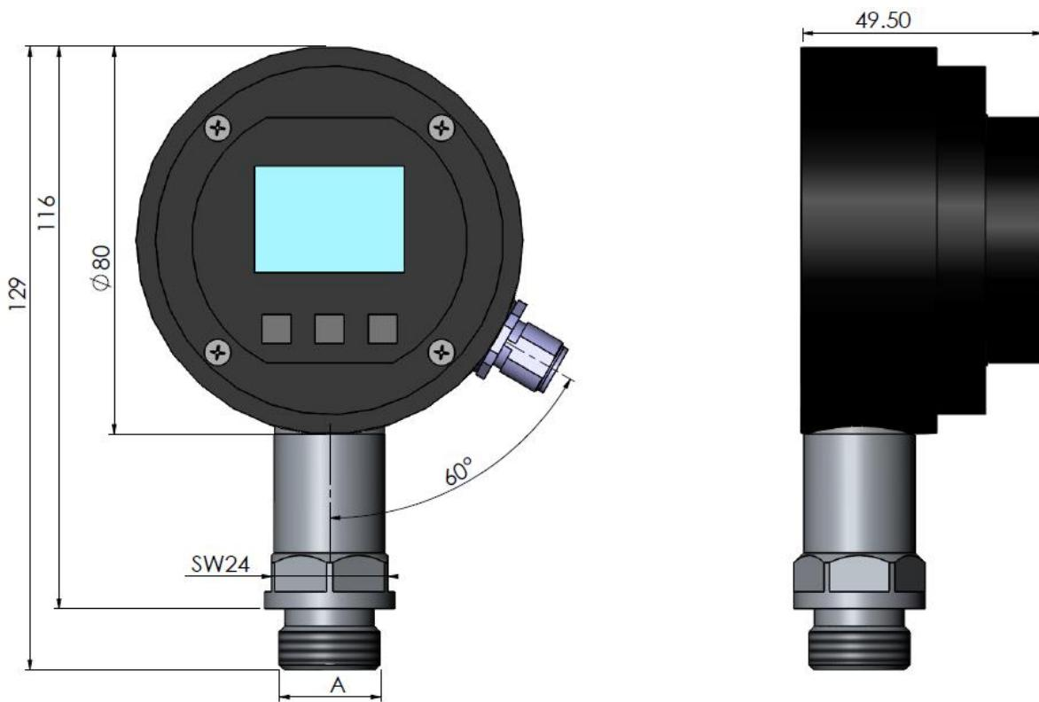
\* Dimension A is the thread dimensions on the pressure sensors.
