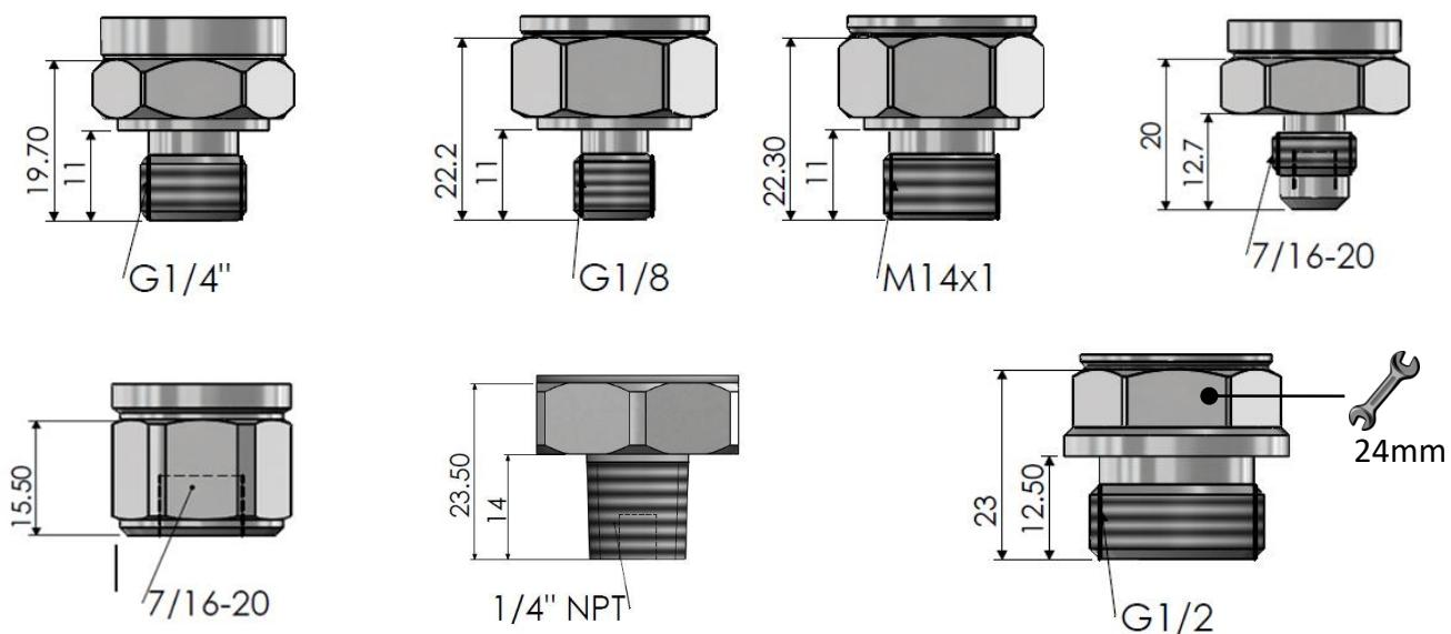
\* In the case of the G1/2 model, the dimension of key slot is 24mm. All other models are 22mm.
