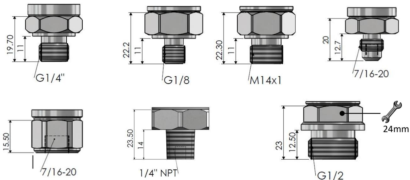
\* In the case of the G1/2 model, the dimension of key slot is 24mm. All other models are 22mm.
