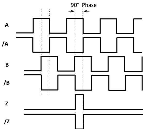
The table above shows the cable colors of the sensor output signals. If the control circuit is suitable in the Line Driver sensors of the not output signals (/A, /B, /Z) have to be added to the system. If it is not suitable /A, /B, /Z signal cables must be fixed as insulated separately. Don't forget that these edges have electricity too.
