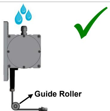
4. The wire should not be pulled in angular. If needed, please use guide rollers.
