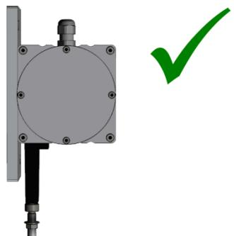
3. If there is a trickle of water (like a rain), the wire outlet must not be a drip of water upstream. If needed please use guide rollers.
