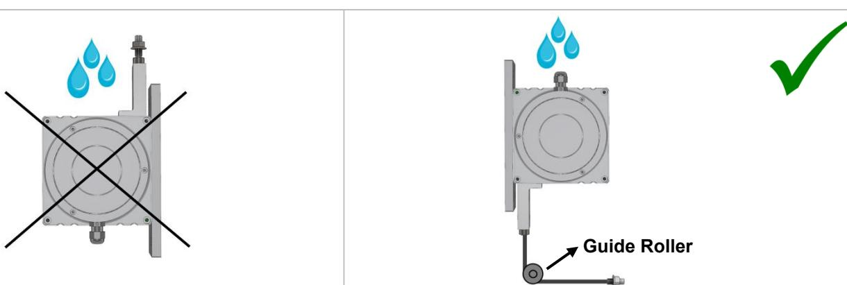
4. The wire should not be pulled in angular. If needed, please use guide rollers.
