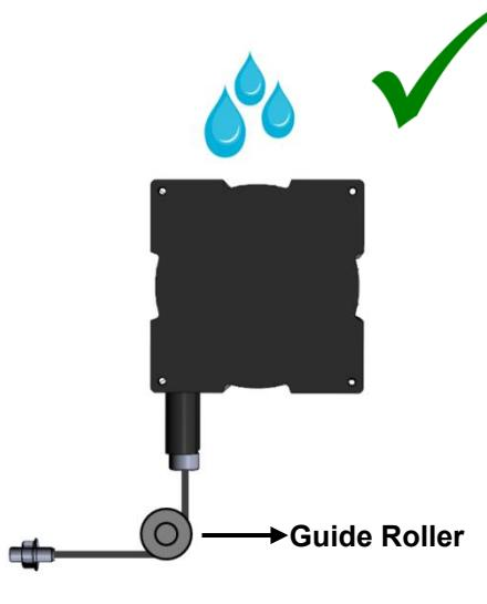
4. The wire should not be pulled in angular. If needed, please use guide rollers.
