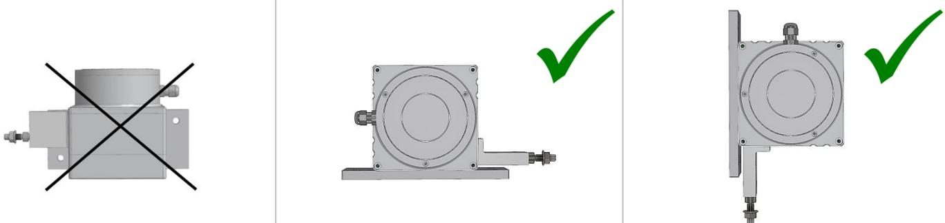
3. If there is a trickle of water (like a rain), the wire outlet must not be a drip of water upstream. If needed please use guide rollers.
