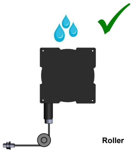
4. The wire should not be pulled in angular. If needed, please use guide rollers.
