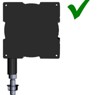
3. If there is a trickle of water (like a rain), the wire outlet must not be a drip of water upstream. If needed please use guide rollers.
