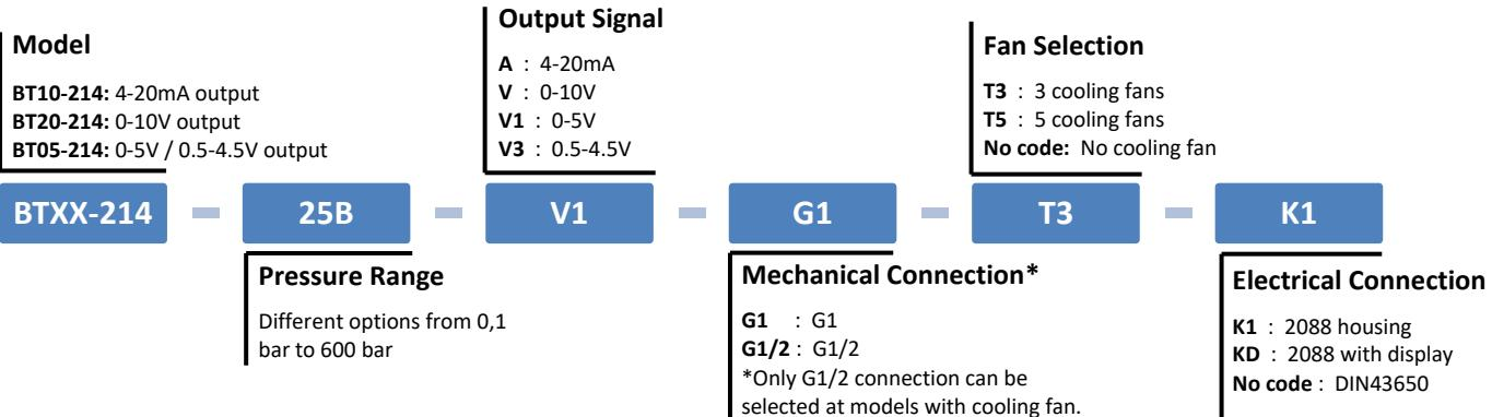
**Note:** Products are supplied as **Gauge** type by default. If **Absolute** or **Sealed Gauge** types are required, this must be specified at the time of order.
