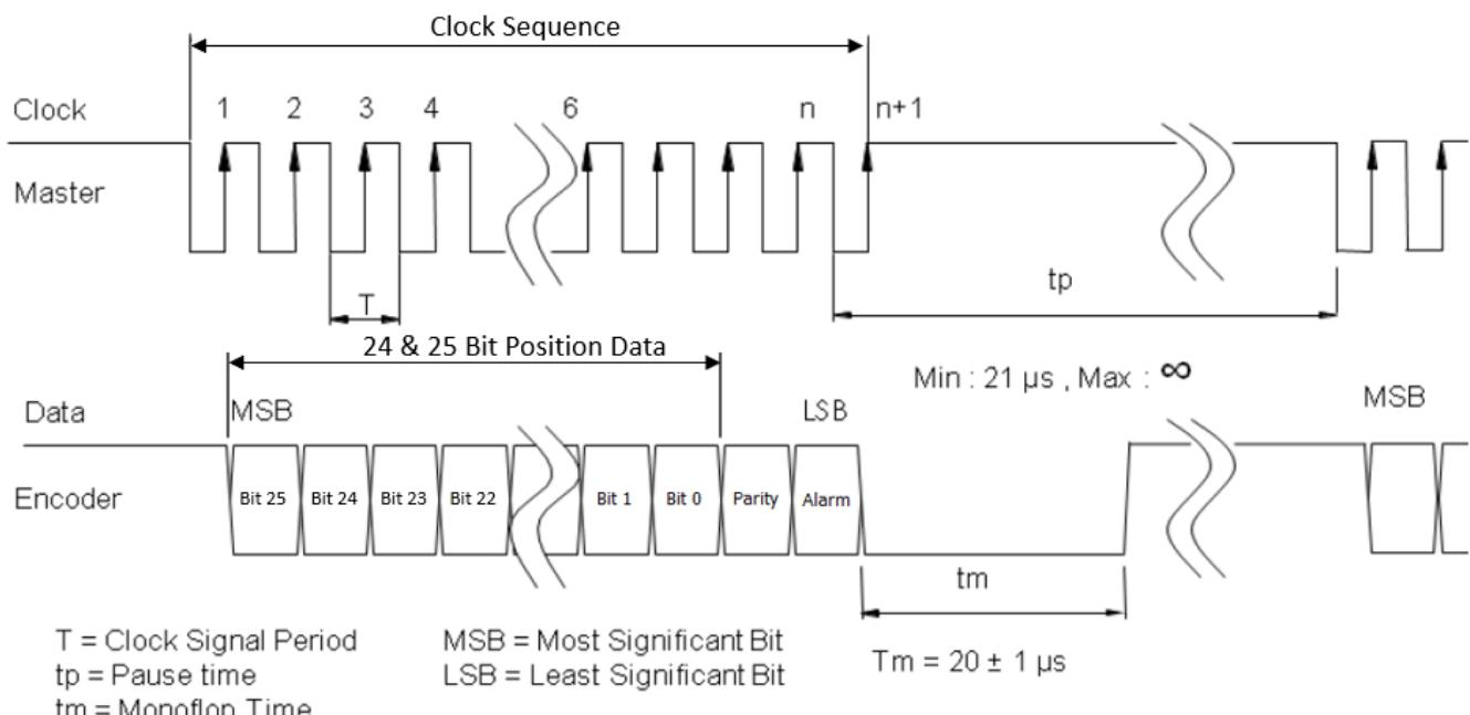
If the device resolution is less than 24 or 25 Bits, the remaining bit fields from the MSB are filled with 0.
